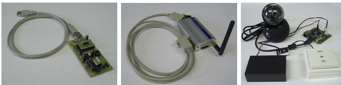
Figure 3. Output devices (USB remote IR TV control, RS232 GSM modem, LAN entrance door system).
