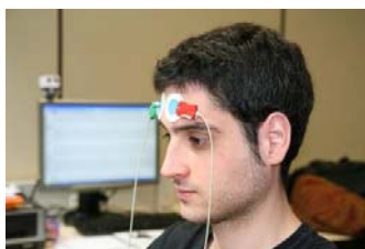
Figure 2. User wearing two electrodes on the forehead and one electrode on the wrist
