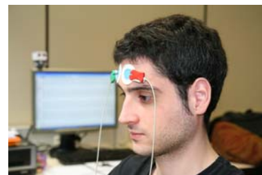
Figure 8. Two electrodes are placed on the forehead to detect muscle activations when raising the eyebrows or tighten the jaw.
