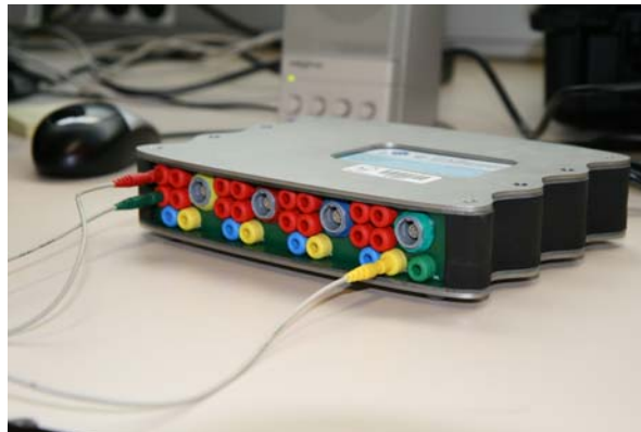
Figure 9. The electrodes are connected to amplifier inputs. The color code corresponds to Figures 7 and 8 to differentiate the ground from the detection activity electrodes.
